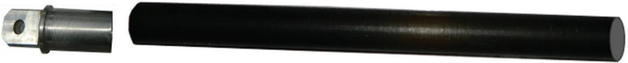
Figure 1. Photographs of CFRP tube (right) and metallic end fitting (left)
