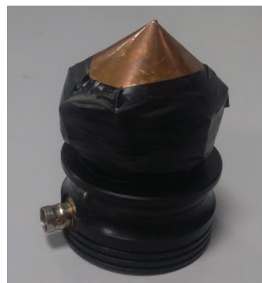
Fig. 7: Photograph showing the conical horn attached to the transducer.
