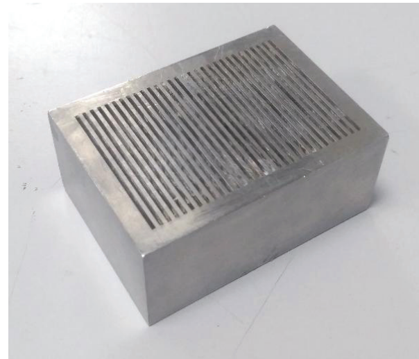
Fig. 1: (a) Schematic illustration of the problem considered and (b) Photograph of the 1D metalens used for imaging.
