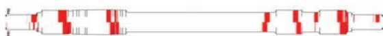
Figure 1: Output for the axle inspection. Indications highlighted in red from the calibration axle.
