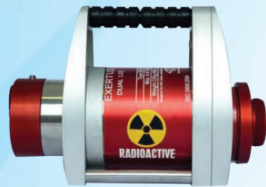
Ir-192 & Se-75 compatible Projector
