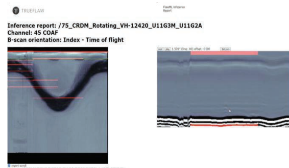
Figure 3: Indications highlighted by the ML model
