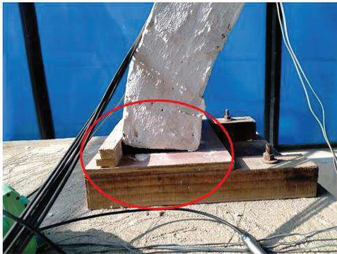
Fig 9 (a) Hinge formation at Fixed End of the Arch
