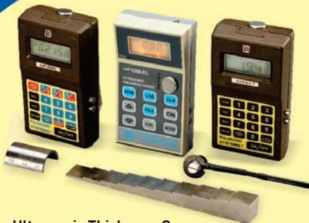
Ultrasonic Thickness Gauges
