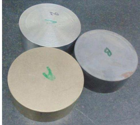
Fig.3: AE961W specimens
