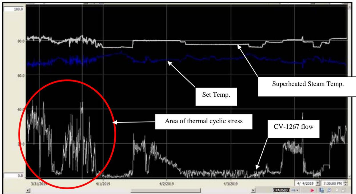
Figure 5 : Thermal Cyclic Stress in Attemperator Nozzle
