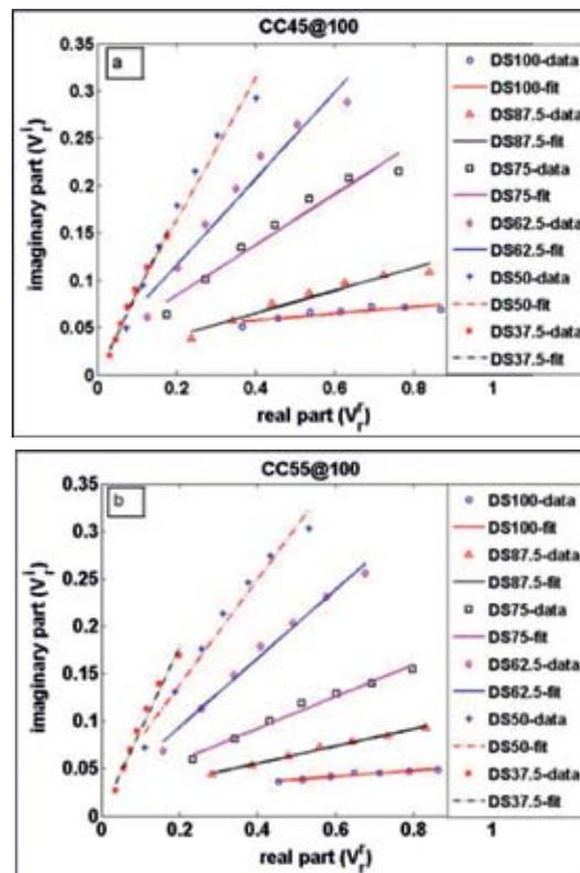
Figure 3 : Polar plot of real vs imaginary parts of voltage ratio  $V_r^i(\omega)/V_r^i(\omega)$  under various DoS and their linear fit along the length for a) CC45 and b) CC55 at excitation frequency 100 kHz
