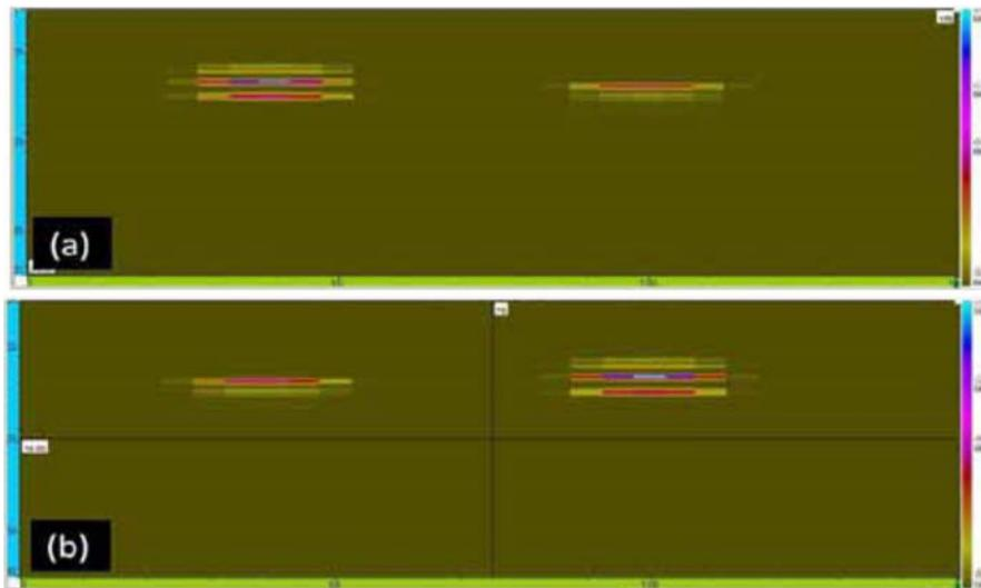
Figure 7 : Simulated B Scan images of DMA probe (LW) scanned from (a) P91 side and (b) Alloy 800 side
