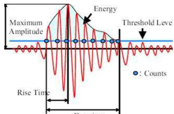
Figure 2 : Parameters involved for acquisition of information from acoustic emission
