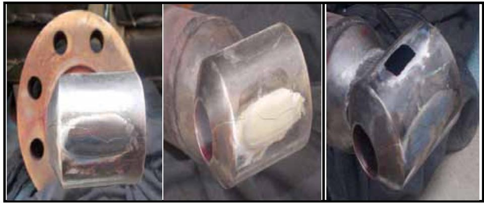
Figure 2 : Surface preparation, Etching And Replica Generation for DSH Nozzle for in-situ Metallography
