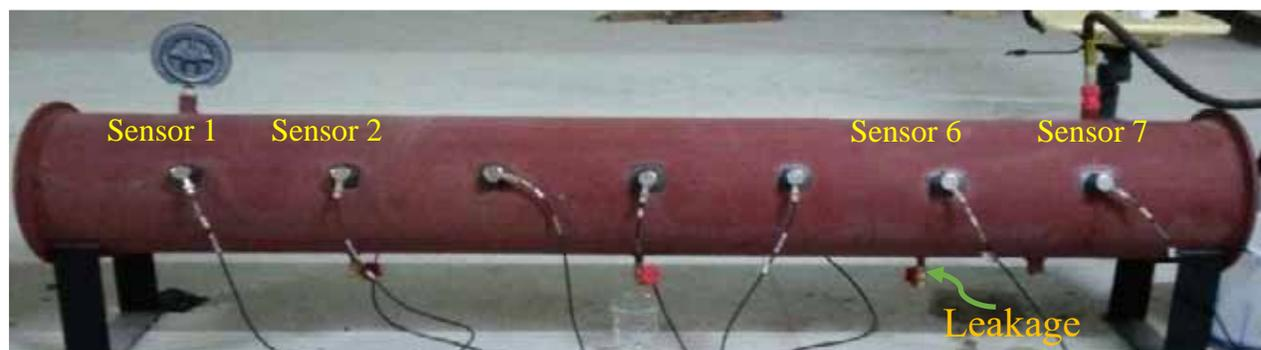
Figure 4 : Experimental setup for leakage detection
