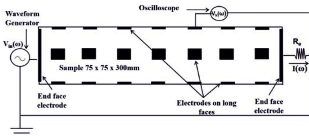
Figure 1 : Experimental set-up [13]
