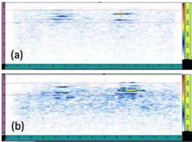
Figure 10 : Experimental B Scan images of DMA probe (LW) scanned from (a) P91 side and (b) Alloy 800 side
