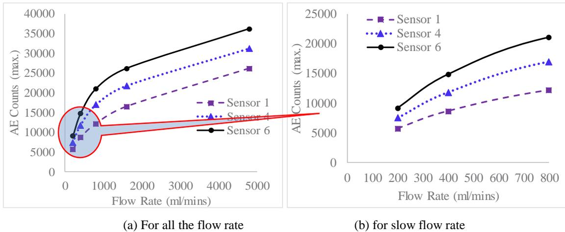
Figure 6 : AE counts plots with respect to flow rate
