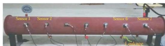
Experimental-setup for leakage detection.
