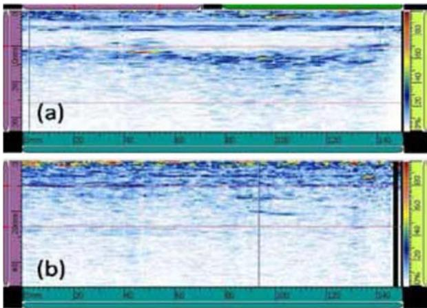
Figure 8 : Experimental B Scan images of LA probe (SW) scanned from (a) P91 side and (b) Alloy 800 side
