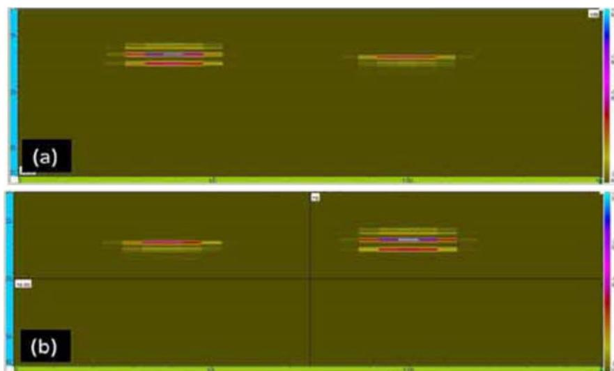
Figure 6 : Simulated B Scan images of LA probe (LW) scanned from (a) P91 side and (b) Alloy 800 side
