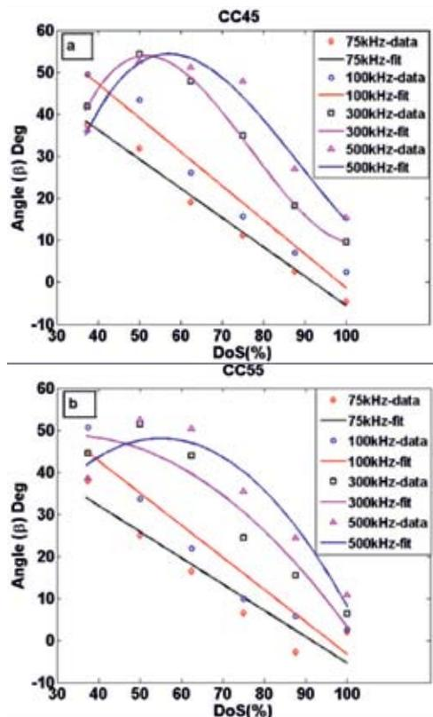
Figure 4 : Variation of angle for estimation of the DoS ( $\beta$ ) under various DoS for a) CC45 and b) CC55 at different excitation frequencies
