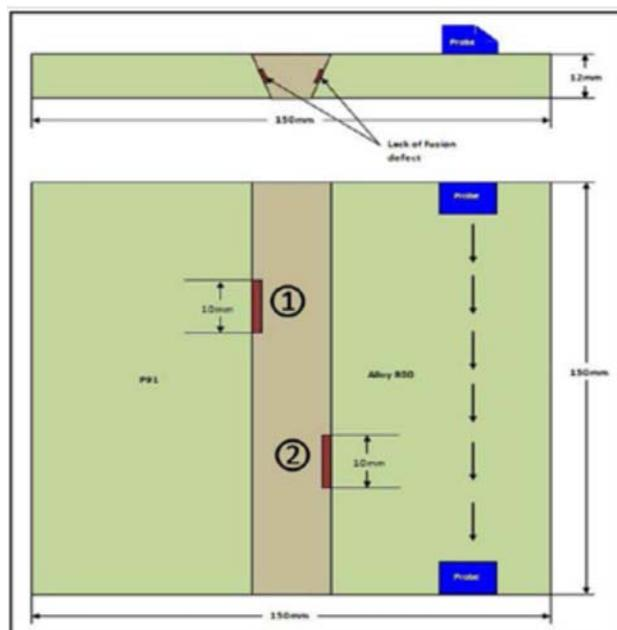
Figure 4 : 2D cad profile of dissimilar weld sample for simulation
