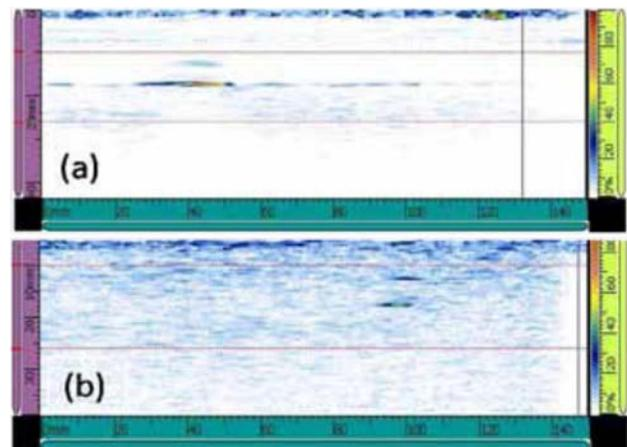
Figure 9 : Experimental B Scan images of LA probe (LW) scanned from (a) P91 side and (b) Alloy 800 side
