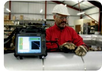
Corrosion Under Insulation By PECT
