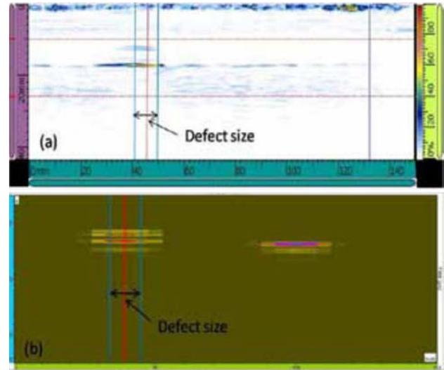
Figure 11 : Defect size calculation by 6dB drop method
