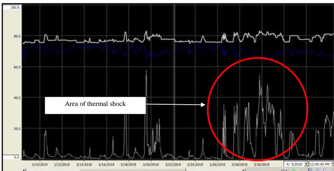
Figure 6 : Thermal Shock in Attemperator Nozzle
