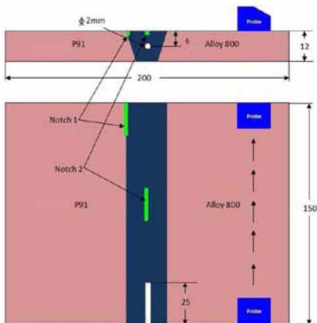
Figure 2 : Schematic diagram of weld joint configuration with Side drill hole and Notches
