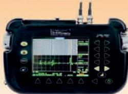
**IMAGING Ultrasonic Flaw Detector**
