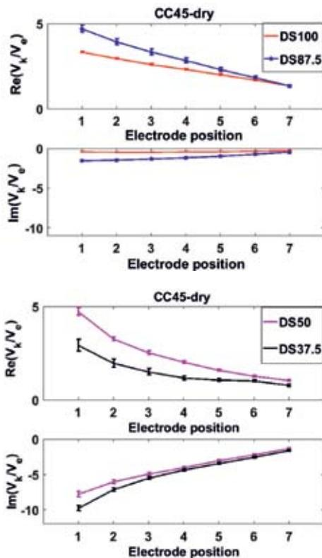
Figure 2 : Error bar showing the spread of 95% confidence interval of real and imaginary parts of the ratio of output voltage and the voltage across the resistance ( $V_k/V_e V_k/V_e$ ) at 300 kHz frequency for CC45 sample
