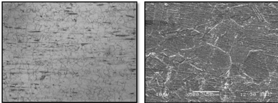
Figure 3 : Matrix's Microstructure at 200X and 500X of DSH Nozzle
