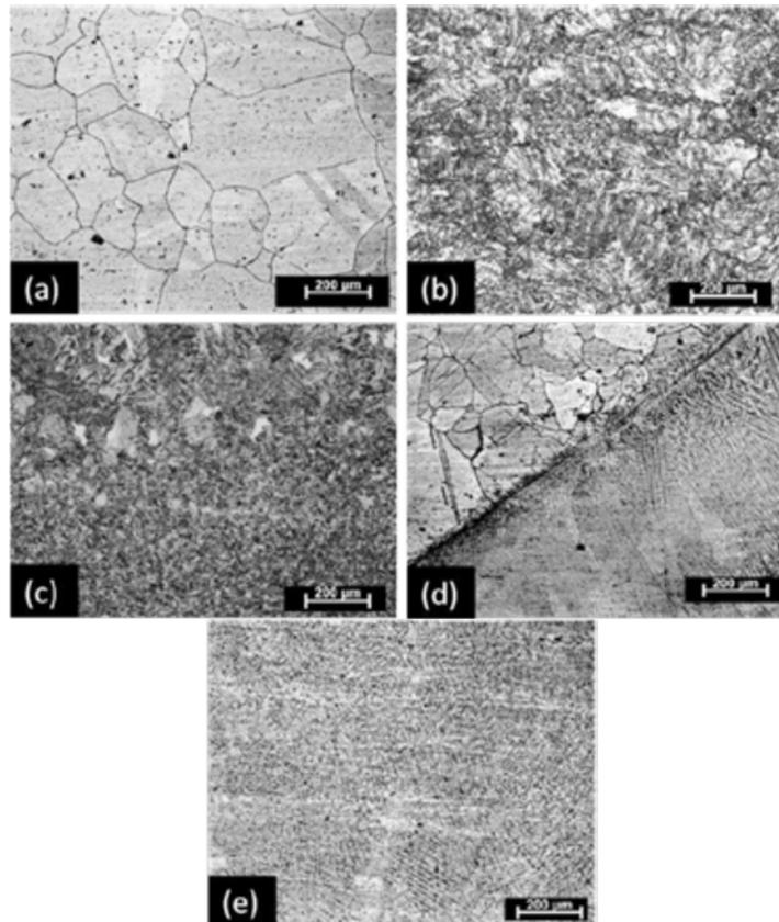
Figure 3 : Microstructure of the Alloy 800 (a) base metal (b) P91 base metal (c) Fusion boundary of P91 (d) Interface of Alloy800 to weld metal (e) Weld metal
