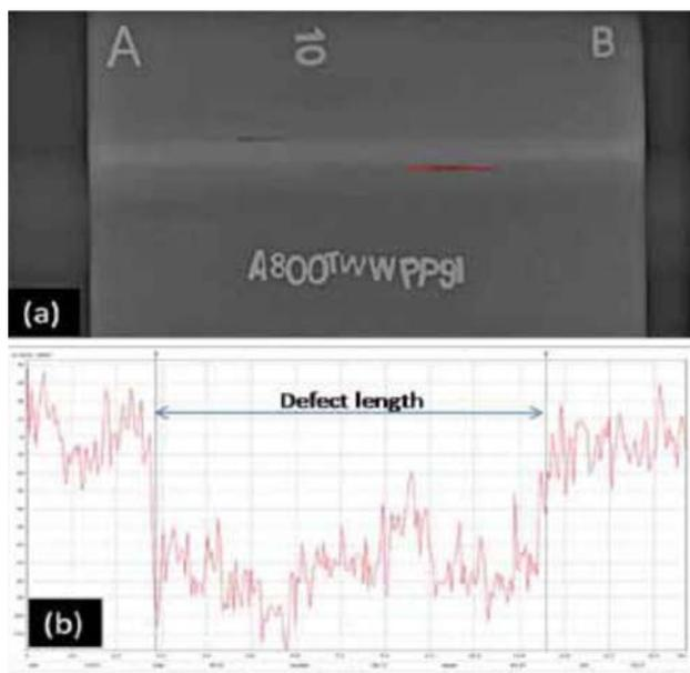
Figure 12 : (a) Radiographic images of dissimilar weld (b) line profile of defect region
