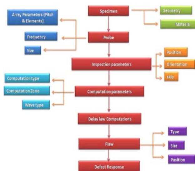
Figure 1 : Flow chart for simulation of ultrasonic inspection
