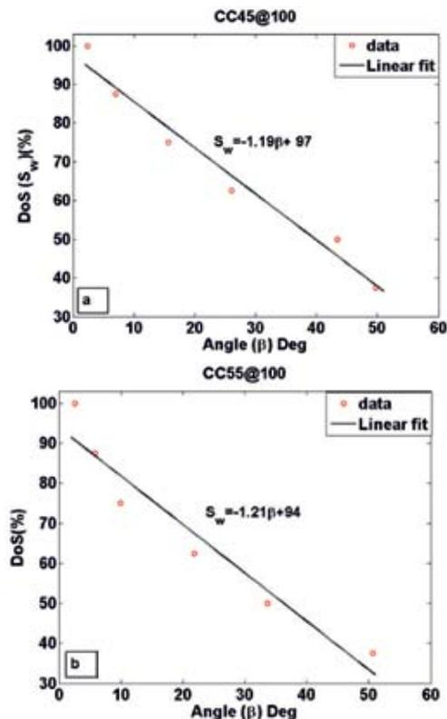
Figure 5 : Relationship between DoS and angle for estimation of the DoS ( $\beta$ ) for a) CC45 and b) CC55 at 100 kHz excitation frequency
