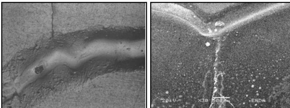
Figure 4 : Microstructure of Crack at 200X and 500X in DSH Nozzle
