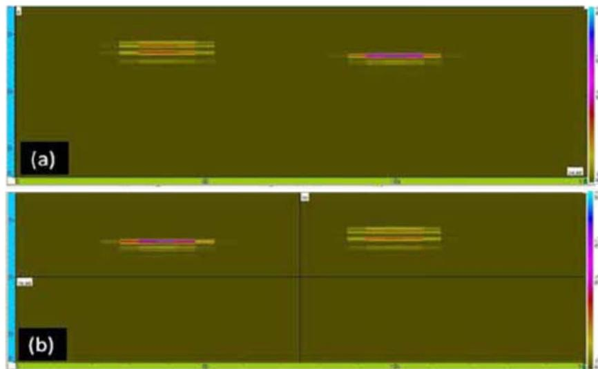
Figure 5 : Simulated B Scan images of LA probe (SW) scanned from (a) P91 side and (b) Alloy 800 side
